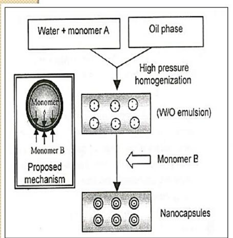
When two reactive monomers are dissolved in immiscible solvents, the monomers diffuse to the oilwater interface where they react to form a polymeric membrane.
